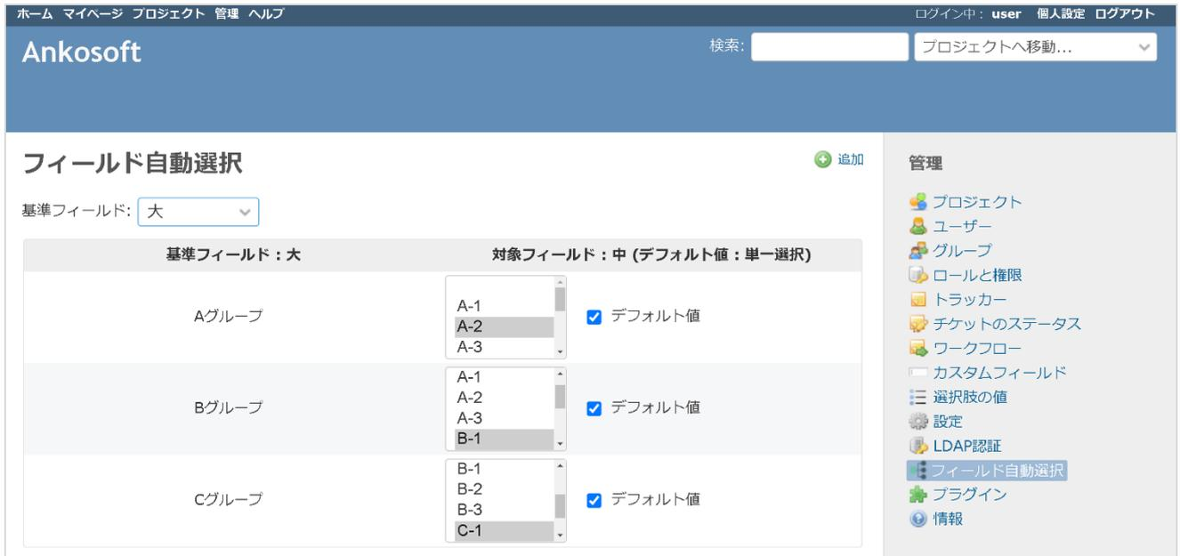
The screenshot shows the 'フィールド自動選択' (Field Auto Selection) configuration page. The '基準フィールド' (Base Field) is set to '大' (Large). The '対象フィールド' (Target Field) is set to '中' (Medium), with a note '(デフォルト値: 単一選択)' (Default value: Single selection). The table below shows the mapping:
